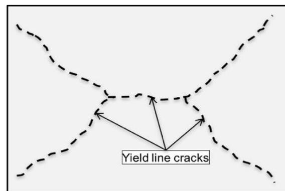
Figure 1 - Fully developed yield line crack pattern
