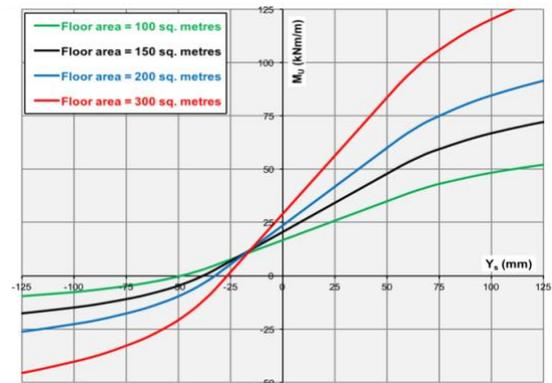
Figure 4 – Effect of floor plan area
