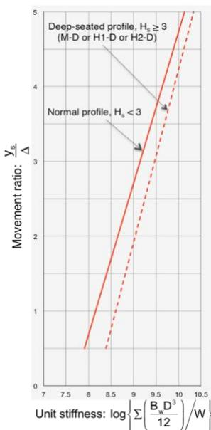
Movement ratio versus unit stiffness
